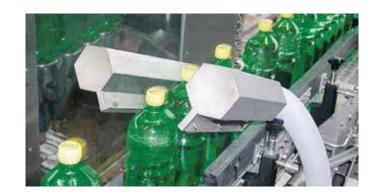
The combination of blow-off nozzles and blowers allows fast and efficient drying of beverage bottles.
