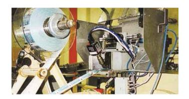
Air heater and blower for drying labels. Fast drying allows for high throughput speeds.
